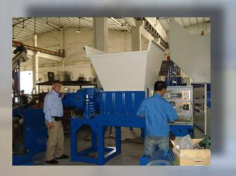
Machines like our 3434, while small, can still shred one ton per hour of various types of solid material. It can be used for everything from preparing light metal scrap to document destruction, hard drive destruction, pre-cut tire shredding and much more.
