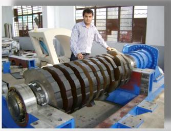
2- The shafts, the blades and the spacers are made from ASTM 4140 HT quench and tempered steel for strength and durability.
