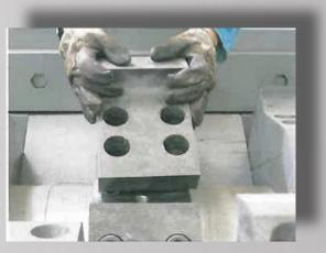
Replaceable blade segments for single man maintanance are an optional extra on machines with blades more than 75mm thick.
