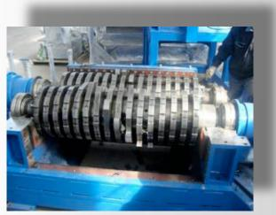
This machines side walls and upper chamber assembly have been removed. The shafts can now be pulled out
