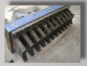
The cleaning fingers are attached to the side wall of the shredder
