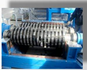
This machines side walls and upper chamber assembly have been removed. The shafts can now be pulled out
