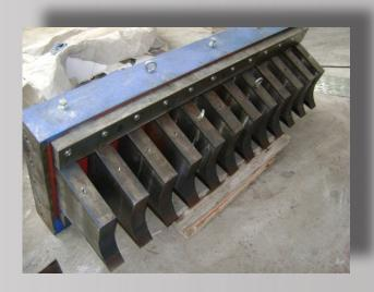
The cleaning fingers are attached to the side wall of the shredder
