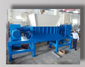
The 5444 is a heavy-duty shear type shredder. The elements that are important for evaluation are the following:
