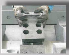
Replaceable blade segments for single man maintanance on machines with blades that are 75mm and above
